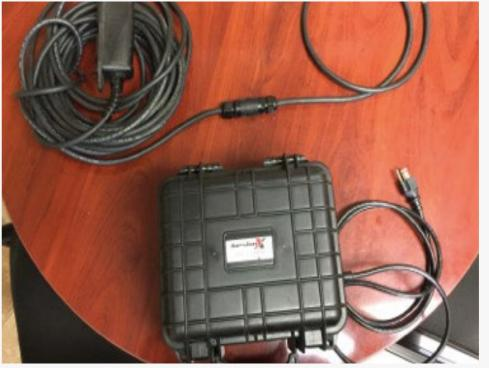
Locking, gender specific cable connections ensure correct attachment and also allow the system to operate in the absence of the intrinsically safe controller (by-pass mode).
