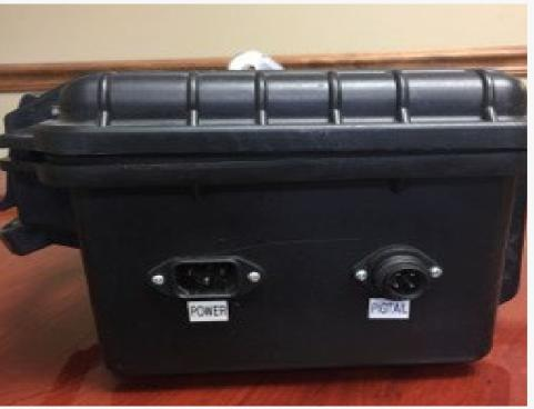
An intrinsically safe controller circuit enclosed in a waterproof polypropylene case, with waterproof connections for wiring to the pump, wiring to the remote hand controller and AC power in.
